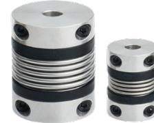
Metal-bellows couplings provide optimum misalignment correction. For the best possible misalignment correction, we recommend torsionally rigid metal-bellows couplings. These couplings feature extremely high torsional stiffness under applied torque and extremely low restoring forces. The clamp fasteners come in two parts for easy and reliable fitting/removal.
