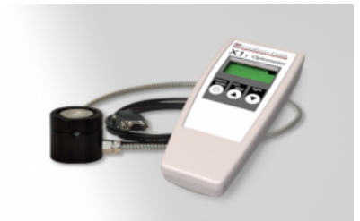
Mobile UV radiometer with separate measuring device and detector for measuring irradiance and dose of 222nm excimer lamps as well as Hg lamps and UVC LEDs.
