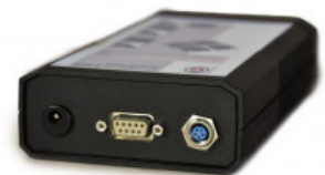
The optometers P-9710 provide connections for power supply, detector heads with calibration data plug and a RS232 interface (from left to right).
