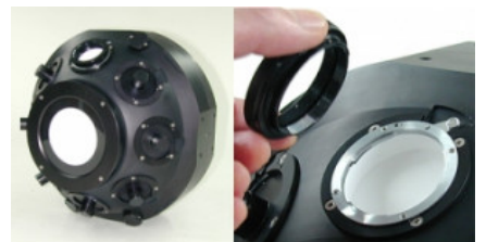
Picture 8: Custom Design 10" Integrating Sphere with Nikon Bayonet Source Mount Adapter
