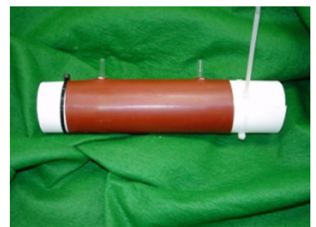
Picture 3: Custom design Integrating Sphere Source Insert
