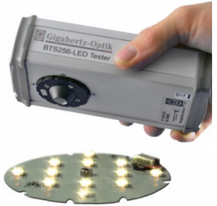
BTS256-LED for measurement of the luminous flux, spectrum, color, and color rendering index of single LEDs
