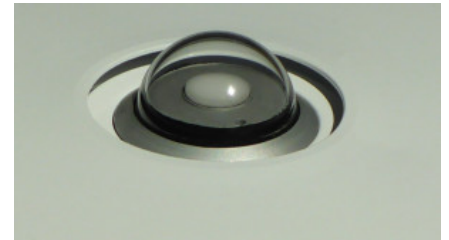
Entrance optic is blow-dried by warm air to prevent dirt, rain or snow
